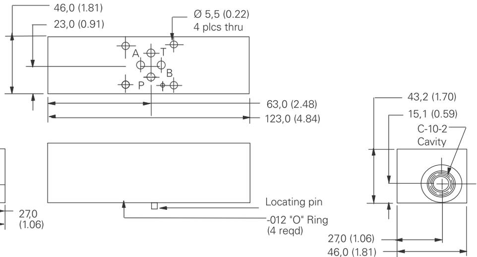
**Note:** This housing may require the use of a spacer block 02-185273 depending upon cartridge valve selection.
