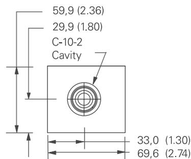
Torque cartridge in housing
