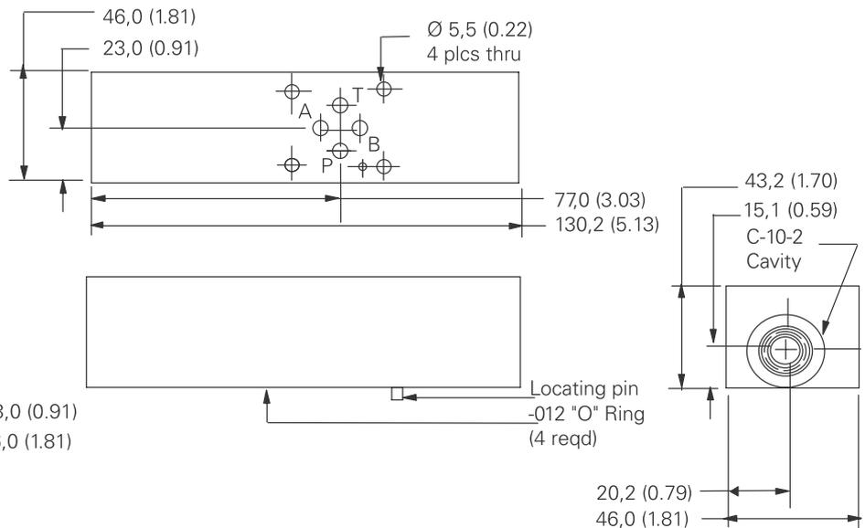
**Note:** This housing may require the use of a spacer block 02-185273 depending upon cartridge valve selection.
