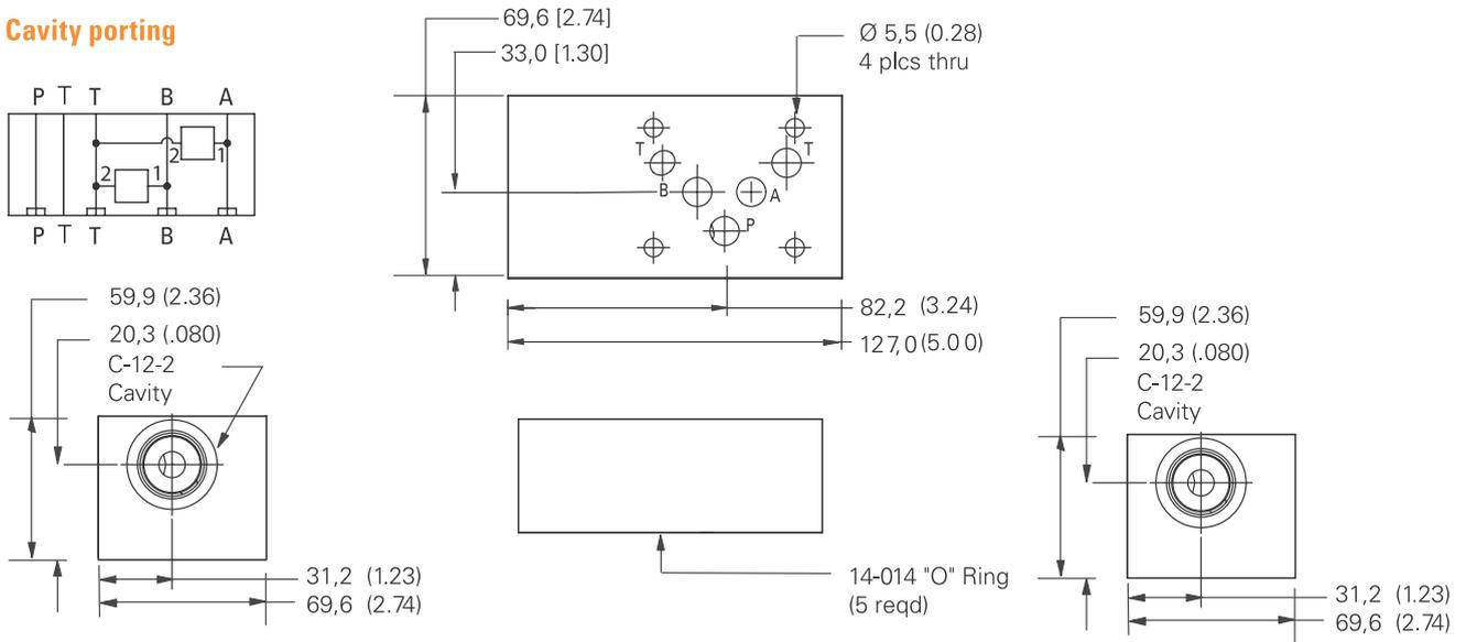
Torque cartridge in housing
