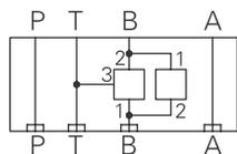
Torque cartridge in housing
