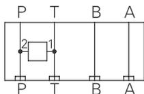
Torque cartridge in housing
