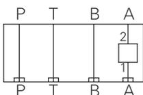
Torque cartridge in housing
