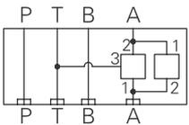
Torque cartridge in housing
