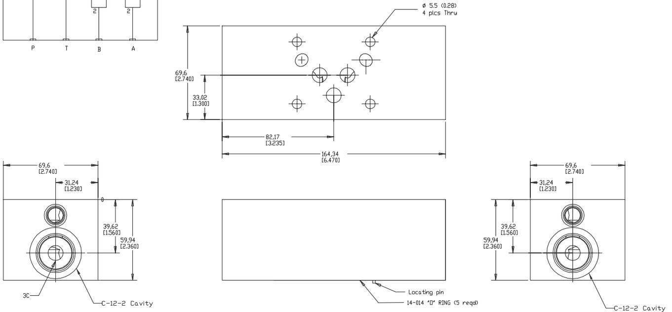
Torque cartridge in housing
