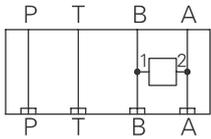
Torque cartridge in housing
