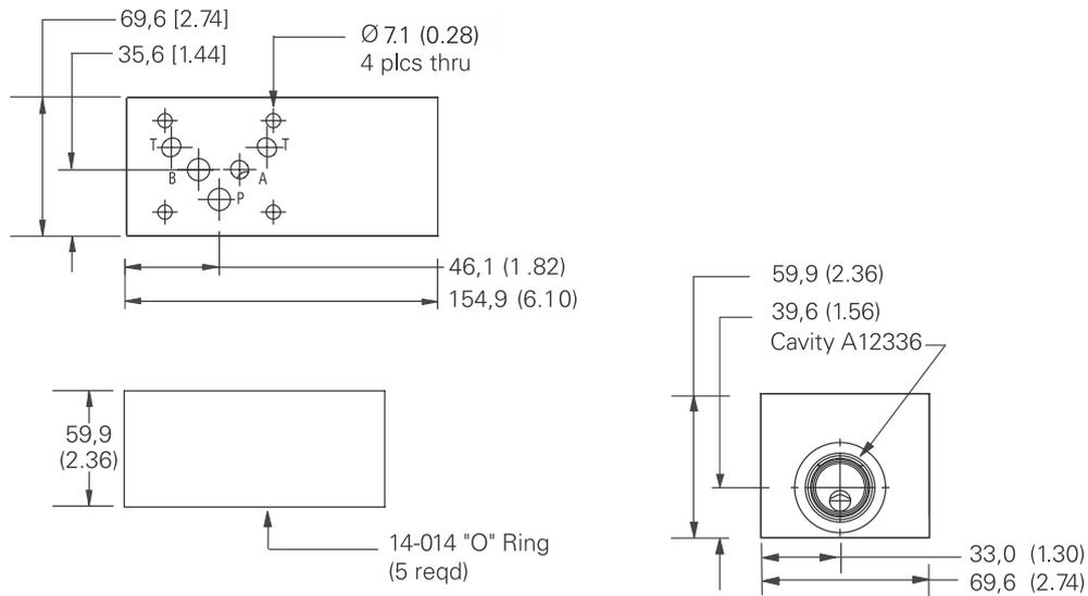
Torque cartridge in housing
