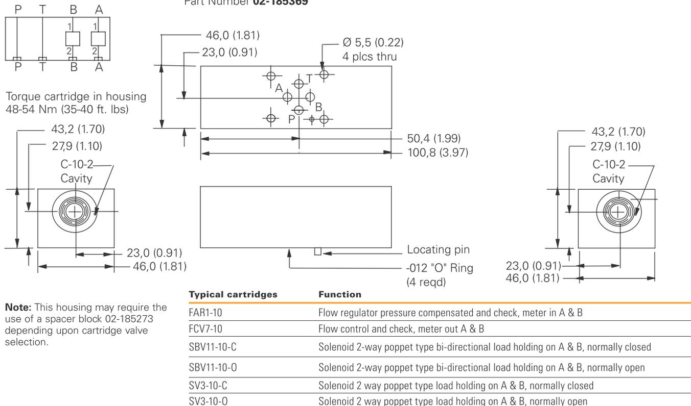
**Note:** This housing may require the use of a spacer block 02-185273 depending upon cartridge valve selection.
